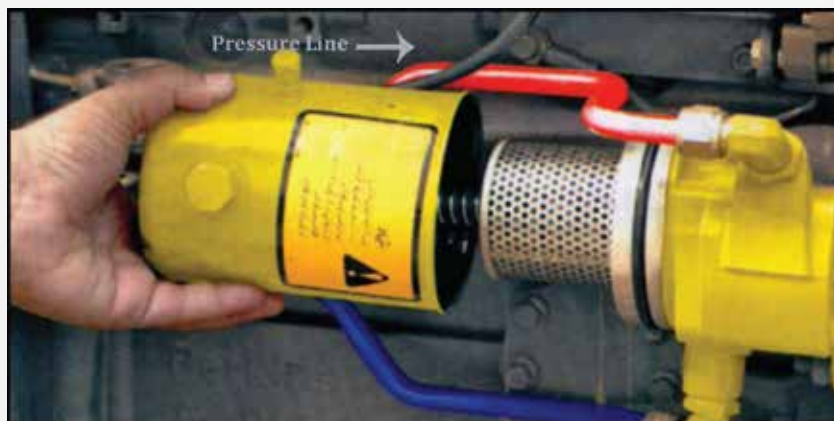
How to change power steering filter MF-385/385 4WD
